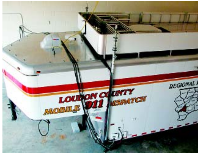
The Gooseneck houses the equipment room. Each corner of the trailer's roof houses a 40-foot extendable mast.
